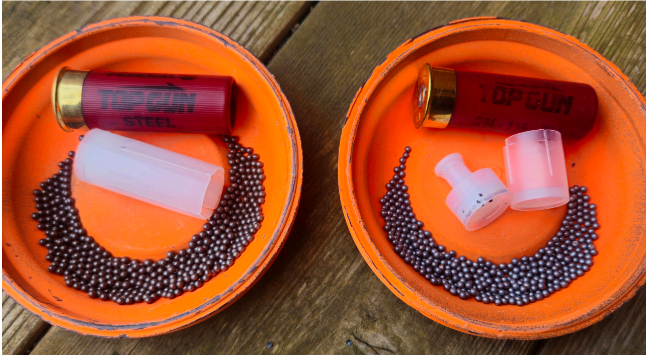
Federal Premium supplied shotshells loaded to the same ballistic specifications. Half contained steel shot (left) and half contained lead, and each material required its own specific shot cup. The steel loads held about 80 pellets more than the lead loads due to steel's lower density.
